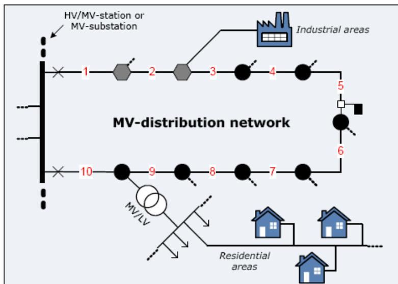
Figure 1. Closed-ring distribution grid with NON (Robert and et al. 2015).
