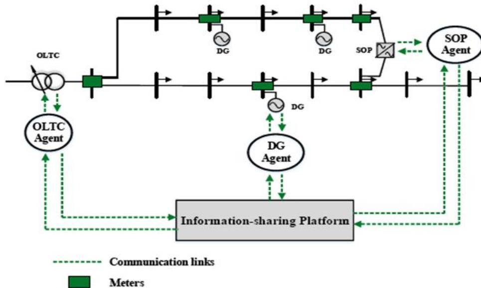
Figure 11. MV grid with online feed back controller to supply power smoothly in abnormal conditions (Fabio Bignucolo et al).
