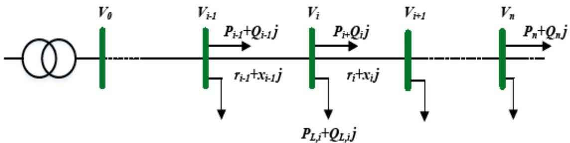
Figure 5. Simplified diagram of one branch MV closed grid.
