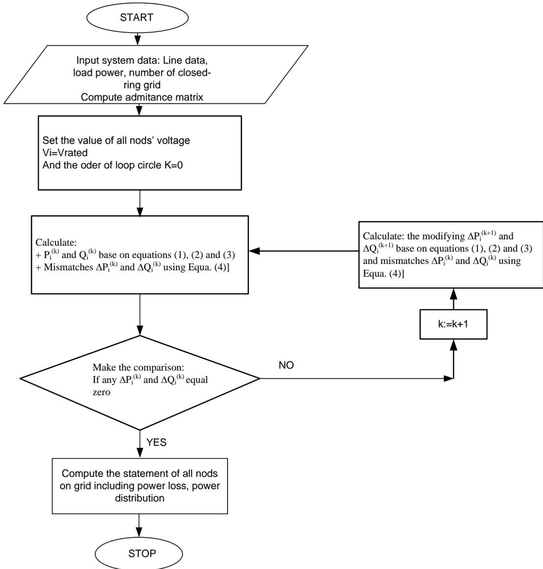
Figure 6: Modified block diagram describing the determining process of NON location.
