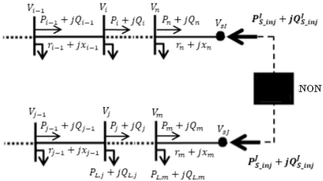
Figure 4. Power distribution in a MV grid with NON.
