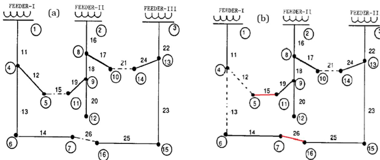
Figure 2. The role of NON in changing the structure of MV grid. (a) Before using NON; (b) After using NON (Wanyu Cao, 2015).
