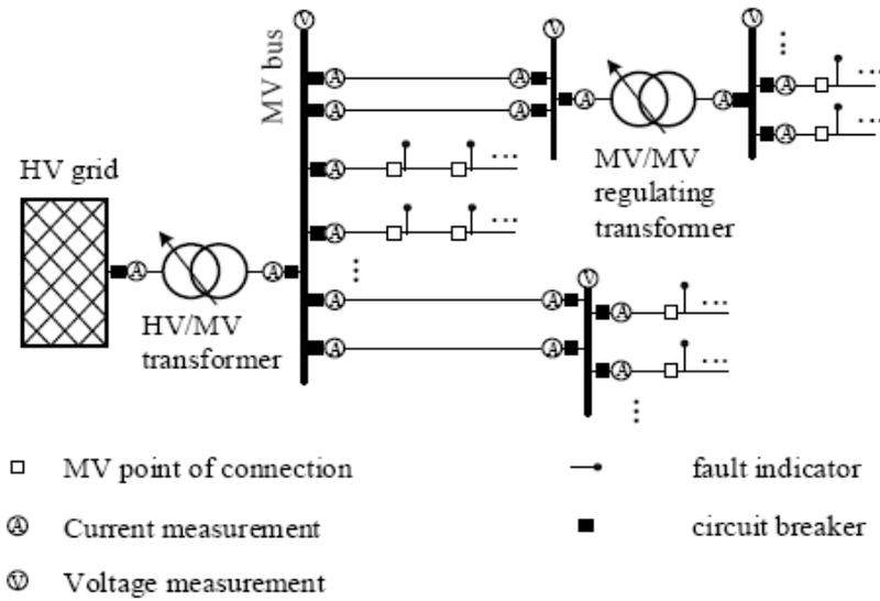
Figure 3. Typical measurement devices in closed MV distribution grid that are not sufficient to locate the NON (Xiang, 2015).
