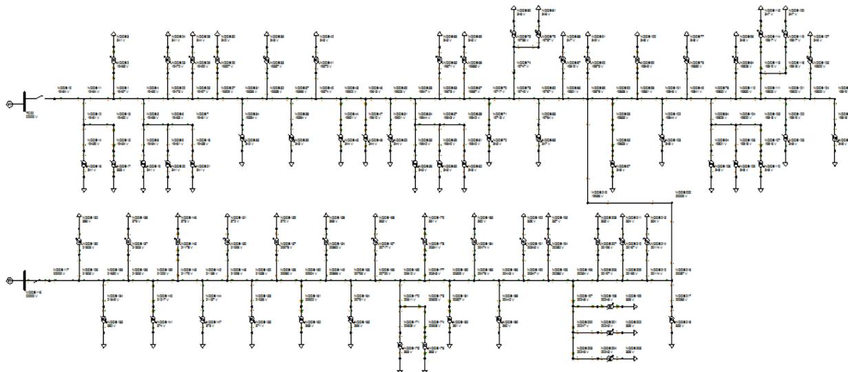
Figure 9. Single line diagram of transmission line No 471 and 474 after being restructured (Dien Bien 22kV MV gird).
